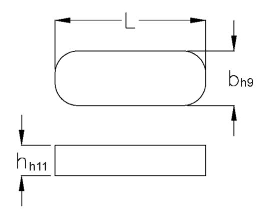
$\begin{array}{ll} b & = 10 \\ h & = 8 \\ L & = 70.0 \\ Tolerance \ b = 0.036 \\ Tolerance \ h = 0.090 \\ Tolerance \ L = -0.3 \end{array}$
